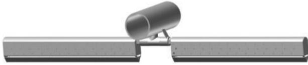
Our Stainless Steel WBCB diffusers are available in 304L or 316L stainless steel. The diffuser is made with cast endcaps welded all around. A typical piping system utilizing SSI WBCB diffusers is made from Stainless Steel pipe with 3/4" FNPT gusseted tees or elbows welded to the bottom center line.
